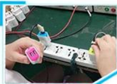
9. Aging test for travel charger
