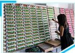
9. Aging test for travel charger
